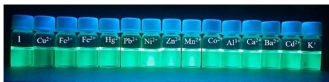
Figure 2. The sensing performance for DTBPA 1 over different cations representing the quenching of fluorescence upon addition of \text{Cu}^{2+} ion.
