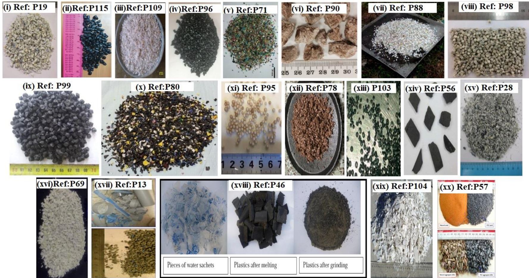
Fig. 2.3 Other polymer aggregates experimented with in literature (Ref: Author index in Table 2.3)
