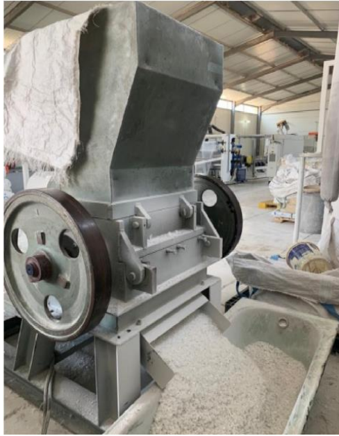
Fig. 3.4 Shredding machine to make PET sand
