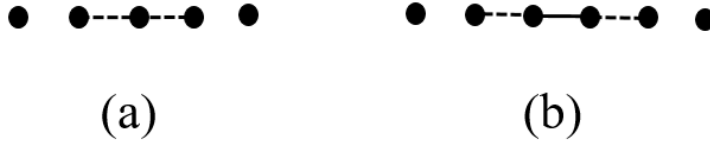
Figure 2.2: Site configuration of the one-dimensional system for cluster size with (a) one site and (b) two sites. The solid line represents the exact hopping within the cluster, and the dotted lines represent the hopping term approximated using the mean-field decoupling \langle \hat{a}_j \rangle + \delta \hat{a}_j .
