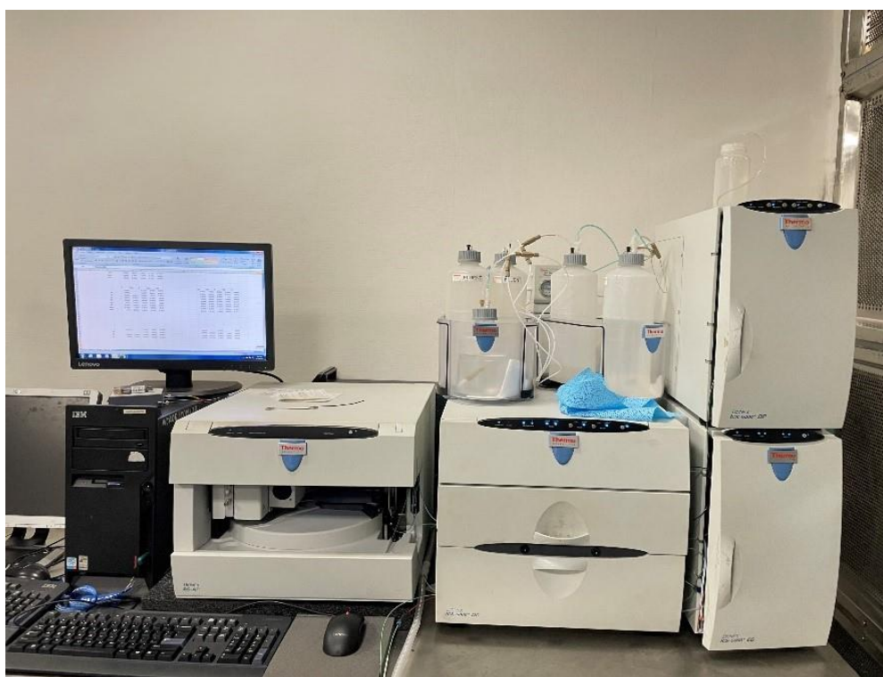
Figure 2.5 Dionex ICS5000 ion chromatograph (IC) used for the measurement of major ion composition in ice cores samples. The IC is housed in a class 100 clean room in NCPOR.
