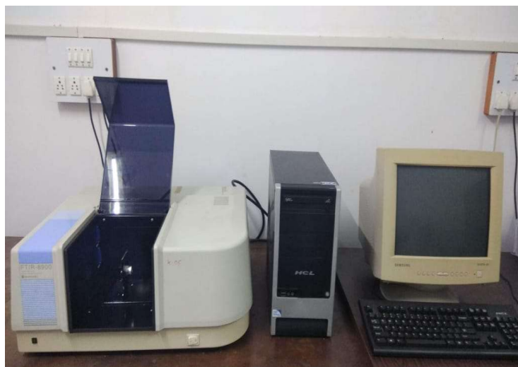
Fig.3.4: Shimadzu FTIR 8900 system, SPAS,Goa university.
