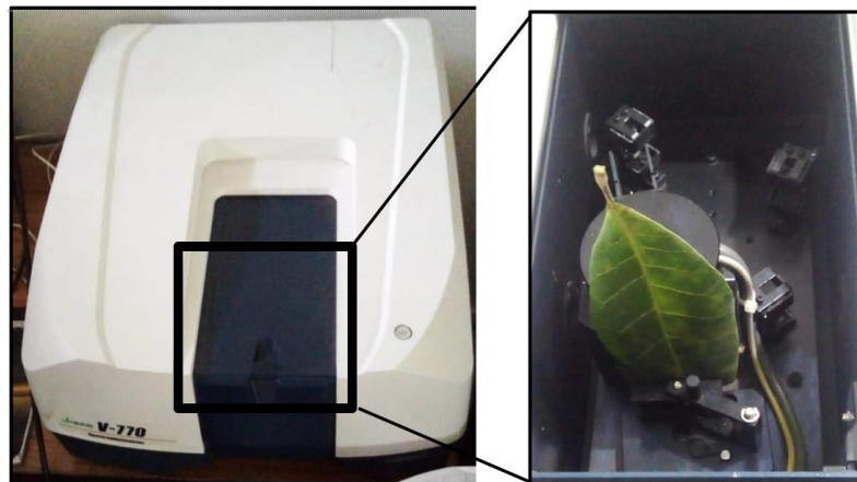
Figure 4.8: Jasco V-770 spectrophotometer, and integrating sphere with leaf
