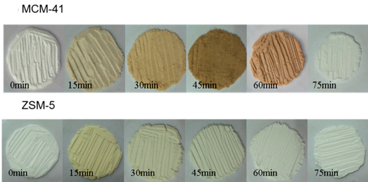
Figure 26. Color changes of the samples during DBD template removal. Reproduced with permission from [110].
