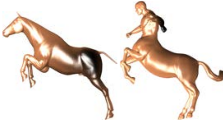
FIGURE 1.4: Partial shape matching between a Horse shape and a Centaur shape from TOSCA dataset (Bronstein, Bronstein, and Kimmel, 2008; Bronstein, Bronstein, Bruckstein, and Kimmel, 2009), where bottom parts of both the shapes match
