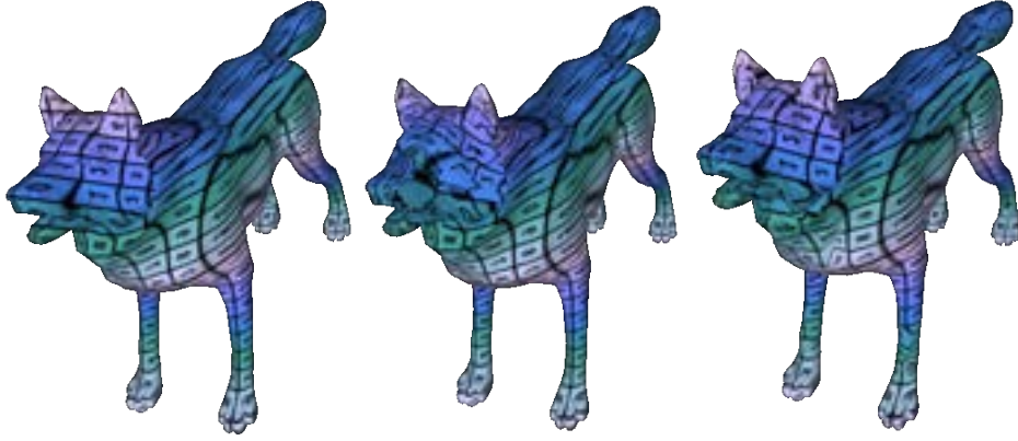
FIGURE 3.7: Texture transfer from one wolf shape to another wolf shape: ground truth map (left), geodesic distances map (middle), and biharmonic distances map (right)
