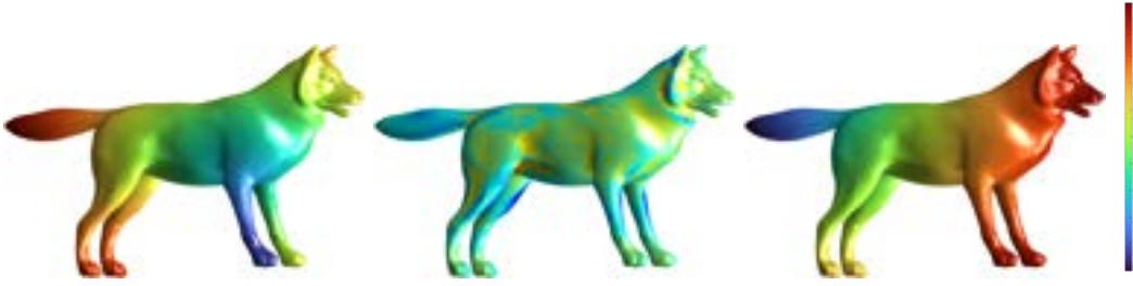
FIGURE 2.4: Visualization of real-valued functions on the TOSCA wolf shape (Bronstein, Bronstein, and Kimmel, 2008), showing geodesic distances from two different source points (left, right) and mean curvature (middle), with blue to red indicating low to high values
