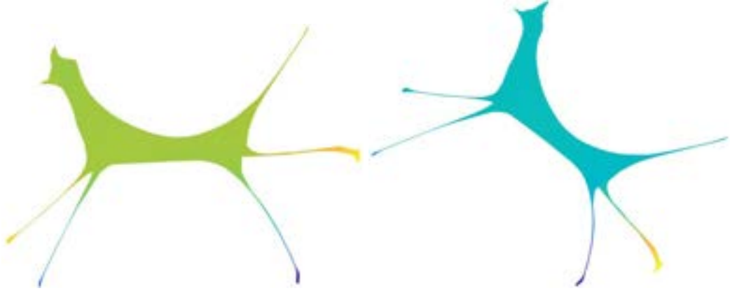
FIGURE 3.3: Canonical Forms derived from Biharmonic Distances for TOSCA wolf shapes (Bronstein, Bronstein, and Kimmel, 2008) via Multidimensional Scaling techniques
