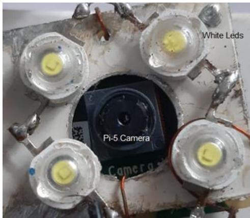
Fig. 6.5c Placement of LEDs
