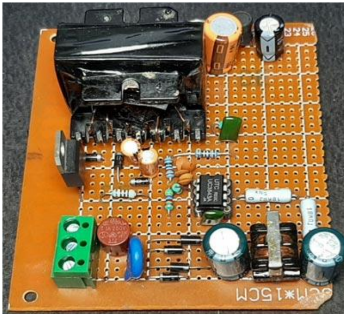
Fig. 6.16 Prototype Power Supply Board
