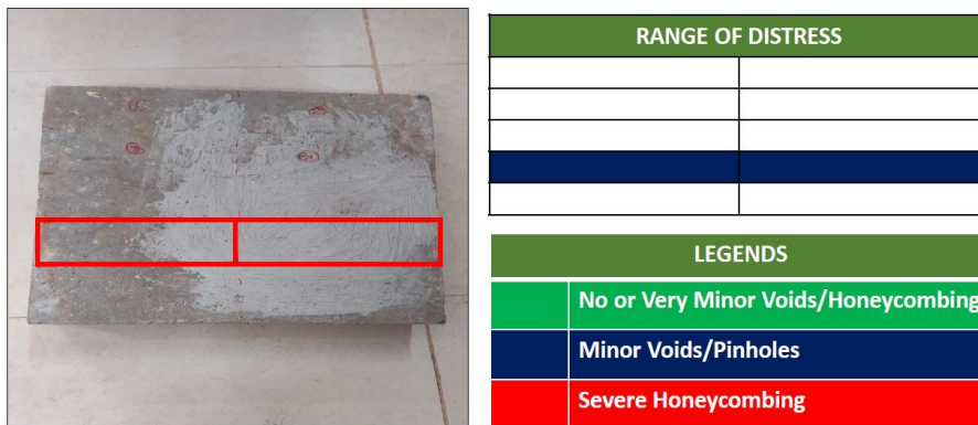
Figure 99 A-scan of surface. Red box shows the extent of area scanned.
