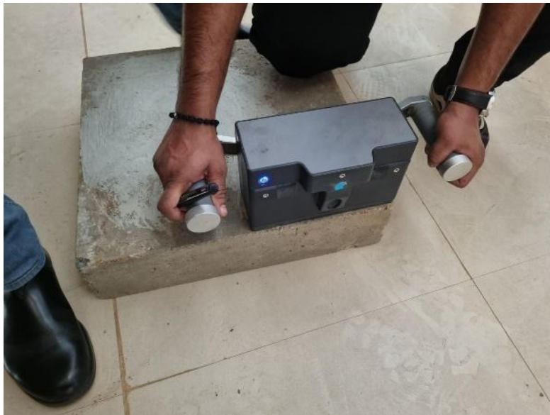
Figure 85 Pundit PD 8050 for CT scanning of concrete slab
