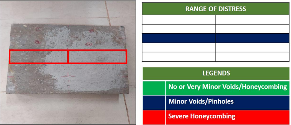
Figure 97 A-scan of surface. Red box shows the extent of area scanned.
