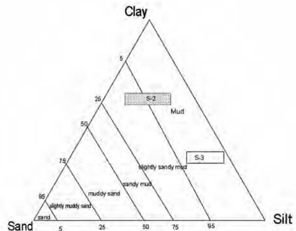
Fig. 3—Ternary diagrams for a revised textural classification of sediments on the basis of sand / mud ratios after Flemming (2000)
